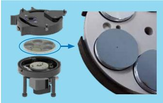
The substrate is either a 1 inch diameter silicon wafer or polycarbonate membrane mounted on a SEM stub. Once the collection surface is conductive-coated the SEM technician can easily find the spot of particles in the exact center of the wafer and measure particle size as small as 5 nm.
