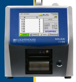
HE SOLAIR 1100LD (Laser Diode) leads the industry as the first of it's kind portable particle counter with 0.10 micron sensitivity and 1.0 CFM (28.3 LPM) flow rate using laser diode technology. Conventional HeNe (Helium Neon) particle counters require frequent cleaning, periodic laser tube replacement and suffer low concentration limits. The SOLAIR 1100LD is designed to operate in ISO class 1 to class 7 cleanrooms without concerns of it exceeding concentration limits.
