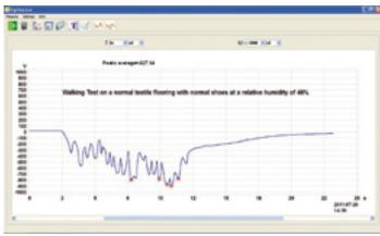
Body voltage measurement test set-up. The new software "Digilloscope" can mark the five highest peaks automatically and calculates the average value.
